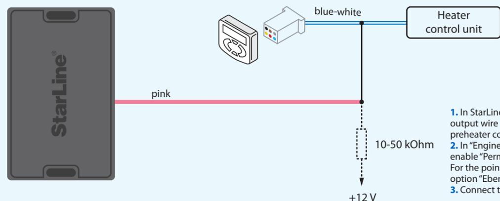
1. In StarLine Master program configure the pink output wire of X3 connector as "Eberspächer preheater control via digital bus"
