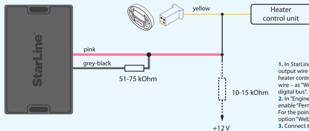
1. In StarLine Master software configure the pink output wire of X3 connector as "Webasto heater control via digital bus", the gray-black wire - as "Webasto preheater start control via digital bus".
