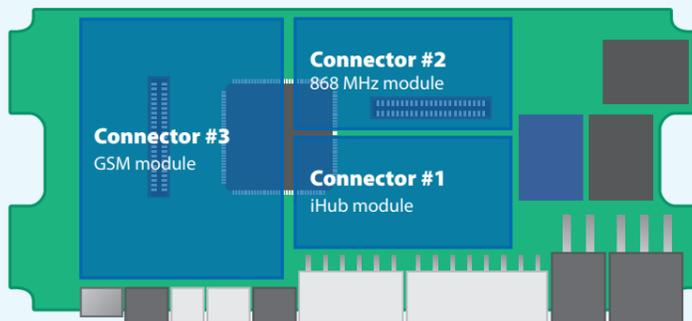
RF 868 MHz module should be installed for system control by means of the remote key. GSM LTE+BT module should be installed to control the system with BLE tag, SMS-commands, via mobile App and at [starline.online](http://starline.online) web account. Analogue channels module should be installed for using the analogue SLAVE.
