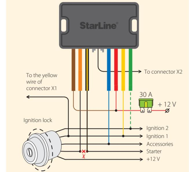
Set X2:6 blue wire as Starter protection and X2:15 orange wire as Engine start: ACC in StarLine Master configuration program.
